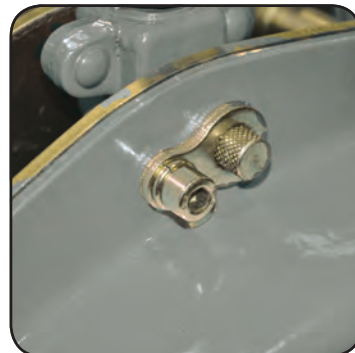
Simple hook replacement due to quick release bolt
